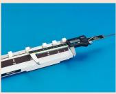
Checking accuracy of caliper (inside measurement)
