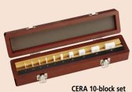
Gauge Block Sets for Micrometer Inspection
