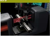
To precisely determine the position of slides on machine tools and measuring devices
