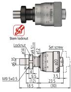
• Fixture thickness: 6 mm Mass: 39 g 148-304 Thimble diameter: 20
