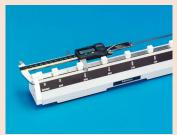
Checking accuracy of caliper (outside measurement)
