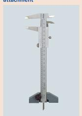
Note: Align reference planes of the depth gage base and extension base using a surface plate and then tighten mounting screws.
