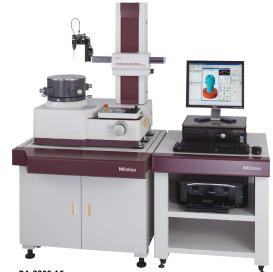
**RA-2200 AS** System vibration isolator (with side table)
